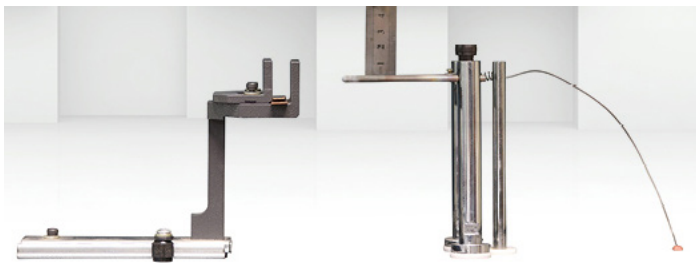
Glow Wire Testing Apparatus Used to Evaluate Different Resins
