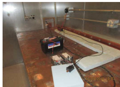
Conducted emission set-up on the power conductor.
