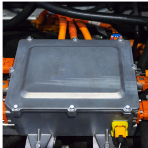
Battery Management System
